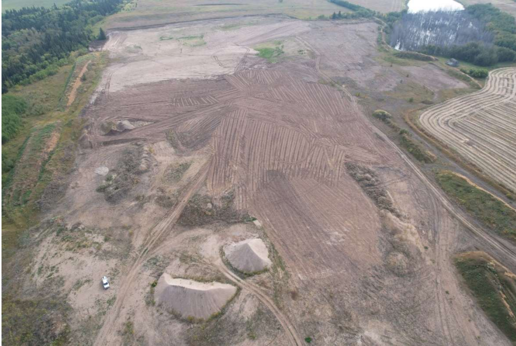
Photo 1: East side of the pit. Waterbody completely backfilled and recontoured. Aerial view (looking east).
